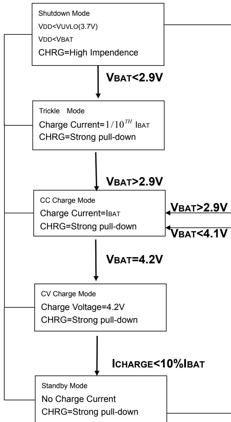
Fig.1 State diagram of a typical charge cycle
